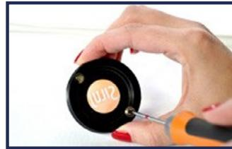
**3.** Unscrew the screws on the gobo holder using a star screwdriver.
