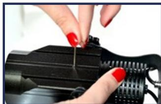
**2.** On the body of the projector, you will find an allen head screw, unscrew it to release the internal gobo holder.
