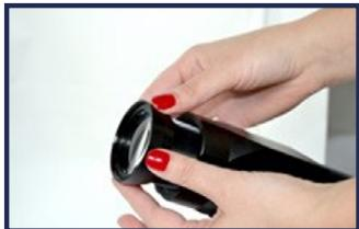
**3.** To make the image clear, rotate the front lens in both directions until the necessary focus is achieved.
