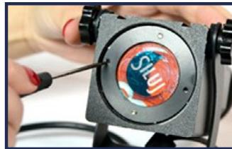
**4.** Place the gobo holder on the thread of the projector body and, using the screwdriver, turn it until it is in the initial position.
