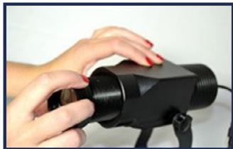
**1.** Unscrew the heat dissipation piece all the way to the end of the thread.
