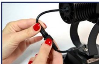
Reconnect the connector that joins the projector body to the base.
