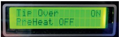
In the ON position (default and recommended), the device stop working if it is roll over
