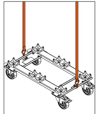
Secure with sufficient lashing straps.
