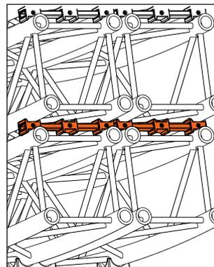
Use Admiral truss carriers to stack the truss.
