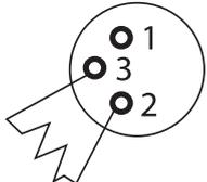
Termination reduces signal transmission problems and interference. it is always advisable to connect a DMX terminal, (resistance 120 Ohm 1/4 W) between pin 2 (DMX-) and pin 3 (DMX+) of the last fixture.
