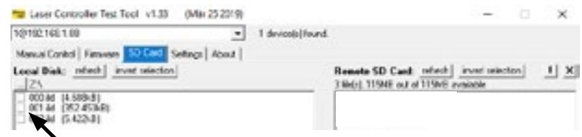
Click on the button with the two arrows to the right to upload the \*.ild files to the integrated SD card. The files are copied and saved now.
