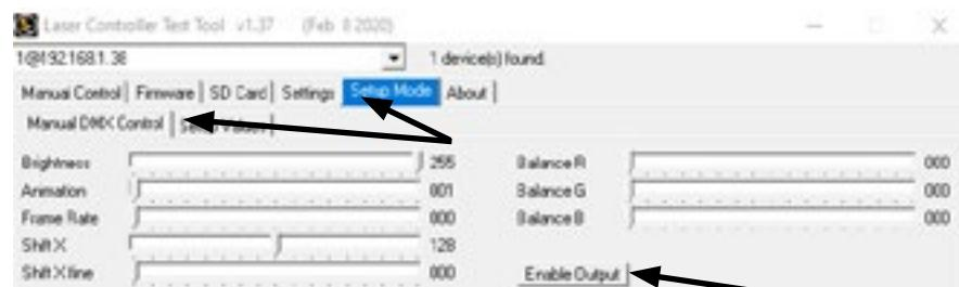
Select the tab 'Setup Mode' -> 'Setup Values' as shown in the picture below:
