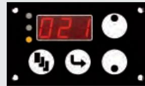
Figure 2: Display when setting the DMX start address
