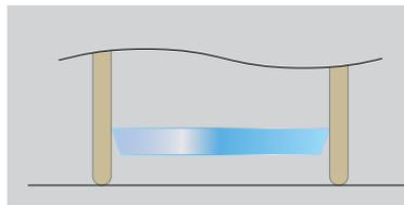
USHIO's UXR unique lamp design protects the front window from surface contact to help prevent scratching and contamination.
