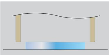
This drawing illustrates window contact on a surface which can cause window scratches and contamination.
