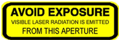
**This laser product is a ClassIIIB laser and has an Interlocked housing.**
