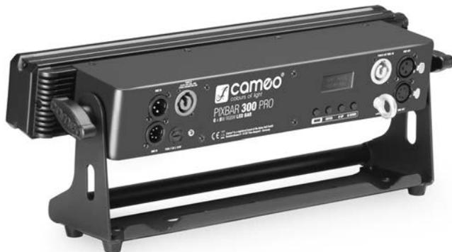
**EN** The Cameo PIX BAR 200PRO, 300PRO and 400PRO can be mounted using the mounting bracket either in a convenient location on the floor or similar, or on a truss system (truss clamp not included). Please use the safety eyelets on the housing to secure the spotlight against falling down. Note: Overhead installation may only be carried out by trained personnel.
